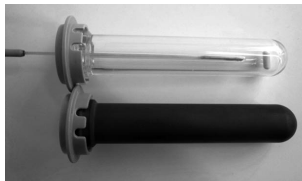
Figure 1. Reaction vial made out of sintered silicon carbide (SiC) for performing microwave chemistry under single-mode conditions. For comparison purposes a standard 10 mL Pyrex vial with a snap cap, internal FO probe sensor and a magnetic stir bar is also shown (see Experimental Section for details).
